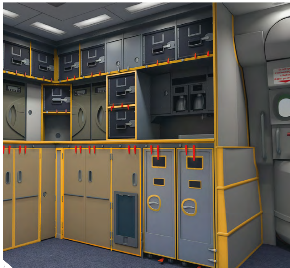
1 Panels assembly, intended for galleys 2 In yellow, application of Sika Products in galley components
