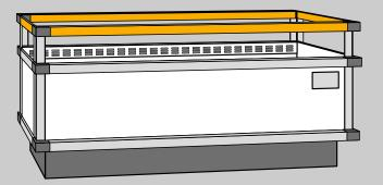
Elastic bonding and sealing of mineral glass on metal frame with **Sikaflex®-260 N**. For applications requiring food approval, **Sikaflex®-522 and Sikaflex®-252** can be used. Reliable assembly of displays and small components in plastics and metals with **SikaFast®-555 L5**. Body removable sealing with **SikaLastomer®-710**.
