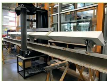
Fig. 4: Fatigue testing on the foam-glass-epoxy ribbons
